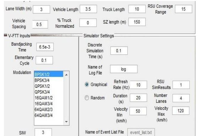
Fig.2: User Interface of the Vehicular Flexible Time-Triggered Simulator (with default Inputs).
