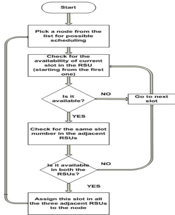
Fig.7: Flow of the VFTT based scheduling algorithm.
