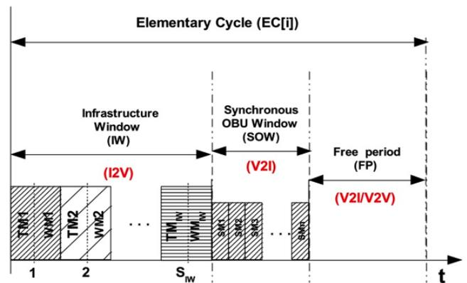
Fig.1: Elementary Cycle of Vehicular Flexible Time-Triggered protocol.
