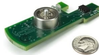
Fig 8: A load cell mounted chip, SMD Sensors [4]
